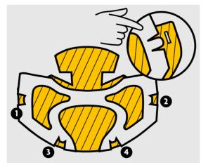
Place the filter on the internal frame following the instruction order in the picture.
