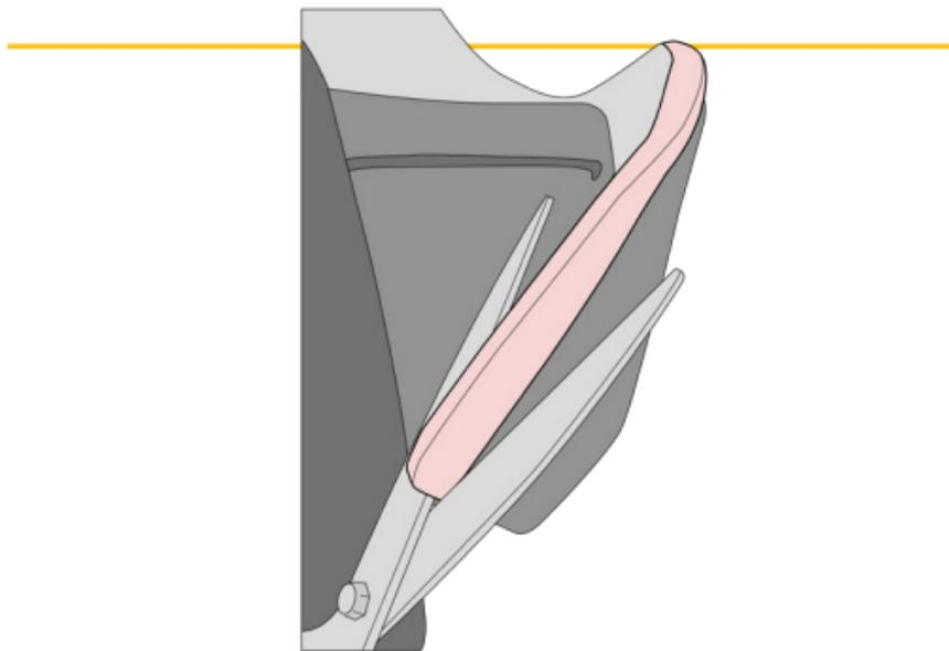
The leg padding must be calibrated according to the tibia, remove any excess material as shown in the figure.
