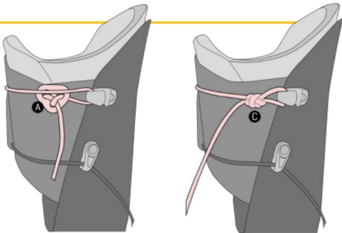
**2. Adjustment of the cuff closure:** It is possible to personalize the cuff closure by adjusting the length of the cord by regulating the knots (outer and inner knot).
